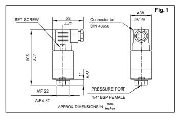
The SA model pressure switches can be mounted in any direction.
